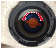
Turn Filters Counter-clockwise to Remove
