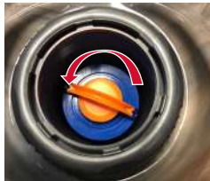
Turn Filters Counter-clockwise to Remove
